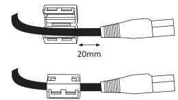
The hinged filter simply folds around the cable and will lock together once you firmly close the shaped channels around the cable. You should fit the filter at the end of the cable as shown. Allow a 20mm length of wire between the plug moulding and the filter. This will ensure optimum performance and allow good cable flexibility.
