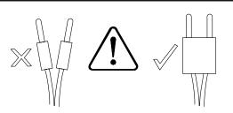
The Power-XR is supplied with a pair of dual speaker plugs. To ensure safe operation of this amplifier, the speaker cables must be terminated with the supplied speaker plugs, assembled in accordance with the instruction supplied with the plugs.
